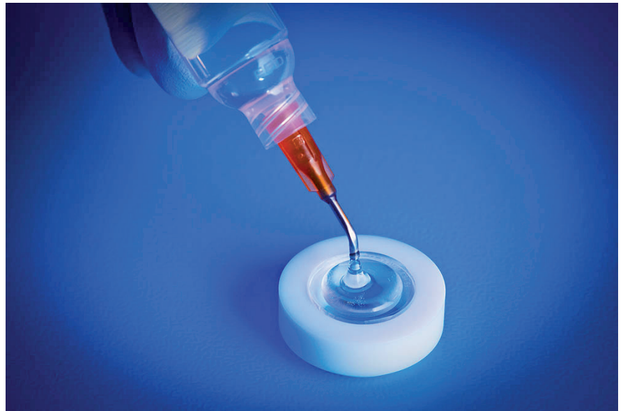
Silicone dispensing during the SENSIMED Triggerfish® Sensor molding process.
